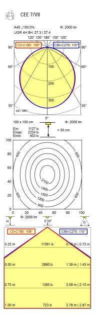
light source LED work equipment electronic transformer connected load 100-240 V, 50/60 Hz; secondary 24 V, DC power consumption env. 30 W luminous flux approx. 2.000 lm luminous efficiency approx. 77 lm/W light type/-color cold white colour temperatur approx. 5.000 K color rendering index CRI > 90; R9 > 50 light distribution direct direct ratio approx. 100 % beam angle 110° chromaticity tolerance LED < 3 SDCM
